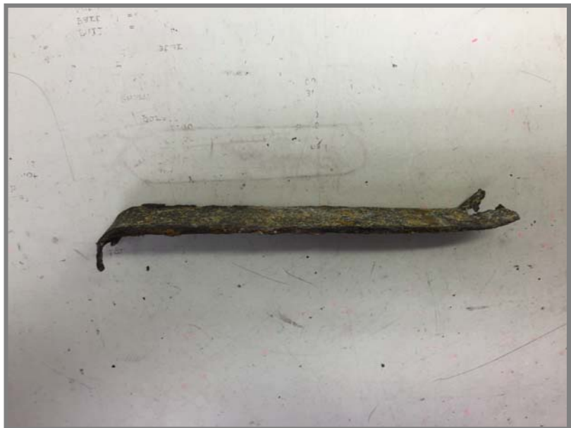
Photo 8 Hooked metal anchor found in mortar joint of cast stone
